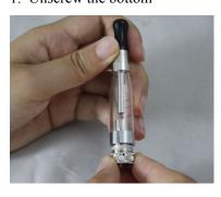
2. Screw off the used coil head
