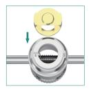
Third, put back the connect pin into the coil base, take out the screw driver and place the heating wire in the middle position, cross pure cotton into the heating wire, make sure the holes are well stuffed with pure cotton and finally cut out spare parts along the holes.
