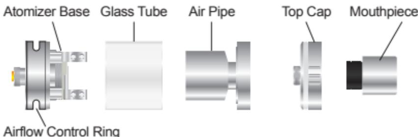
1. First screw off the atomizer base and fix the pre-made or self-built coil with cotton on the atomizer base. (Note: please make sure the finally fixed coils do not come into contact with the surface of the deck and the inner wall of the air pipe.)
