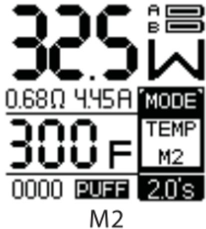
In the temperature control mode to replace the heating wire, the first let Heating wire in the indoor temperature, after installed the heating wire, The screen will appear the heating wire resistance, Figure 1 is the heating wire Of the initial value, if the "resistance" is very accurate directly Use, if not very accurate then need to correct the heating wire Of the resistance.
